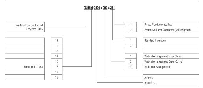
**Example:** Insulated Conductor Rail Program 0815;  $R_2 = 2500 \text{ mm}$ ;  $\alpha = 90^\circ$ ; vertical Arrangement (Outer curve), standard insulation, phase, copper rail 100 A. Part No.: 081516-2500x090x211
