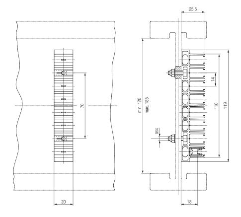
14 mm pole spacing. The 8-pole hanger clamp is shown.
