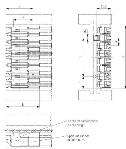
8-pole "End Cap Set complete" without power feed is shown. (8-pole "End Cap Set complete" = End cap set + 8 pcs. end caps for transfer points/end cap "long"). This end cap set is screwed onto the overhead runway beam section. The end caps of the individual conductor rail poles are clipped into it.
